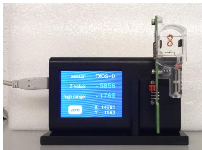
Figure: The MyoDish tester with a chamber containing a test weight.
