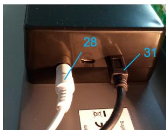
Figure: Controller unit (7) with barrel connector of the power cord (28) and micro-B connector of the USB cable (31) connected.
